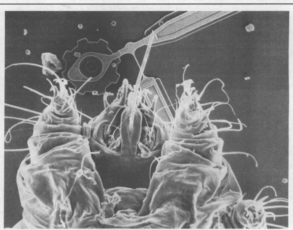
INVASION OF THE MICROGEAR-SNATCHERS? — A dust mite, no bigger to the human eye than a tiny dot, crawls over one of Sandia's micromachines. The machine turns gears, each smaller in diameter than a human hair and one-hundredth the weight of the dust mite, at hundreds of thousands of revolutions per minute. The latest Sandia micromachine is a smart one, incorporating microelectronic "brains." See story on page 5.
